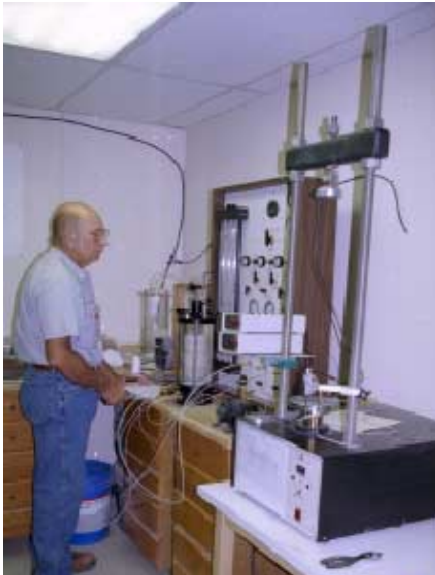
DCE Technician Performing Permeability Test in Geotechnical Laboratory
